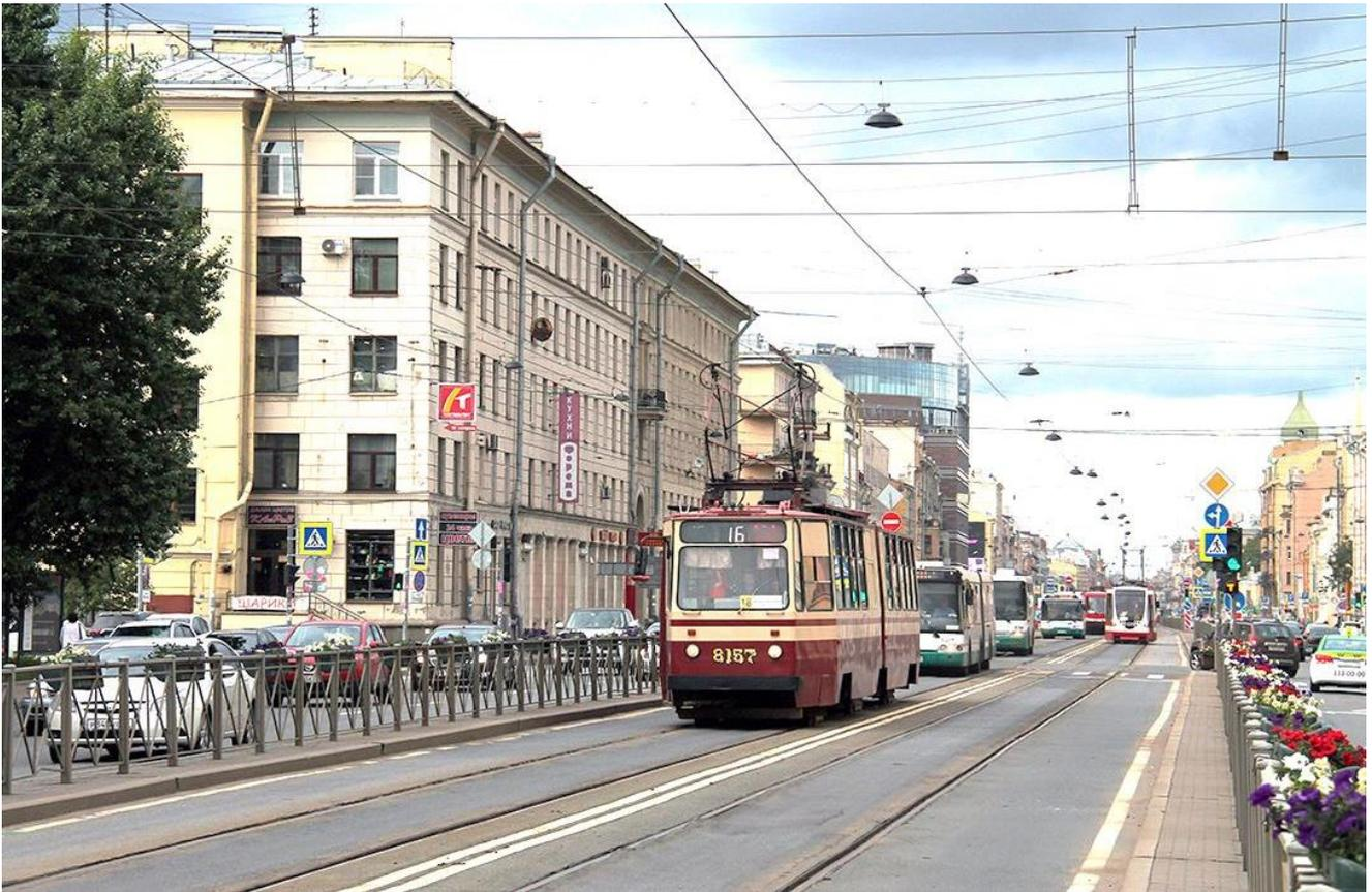
Fig. 5.2. Priority lane for buses and trams in the center of the roadway (Ligovskiy prospect).
